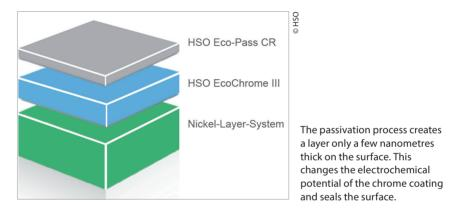
and involves creating a layer only a few nanometres thick on the surface. The passivation process changes the electrochemical potential of the chrome coating and seals the surface. As a result, the coating meets the high standards required by the automotive industry. The trivalent chrome process is more expensive and Willy Remscheid estimates that this leads to a price increase of between 8 and 14 percent, depending on the type of component.
